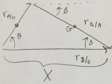
$$r_{A10} + r_{G1A} = r_{B10}$$
