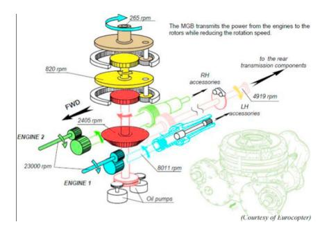
**5.** <u>This paper</u> describes a planetary gear system in a helicopter (see the figure). The ring gear in both epicyclic gears are stationary. The figure shows the angular speeds of the sun and planet carrier on the two systems. Select numbers of teeth for the ring, sun and planet gears in the two epicyclics (find the lowest possible numbers of teeth on each gear).
