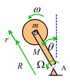
4.1 Suppose that the bar AB rotates with angular speed  $\Omega = d\theta / dt$  and the reaction wheel rotates with angular speed  $\omega$  *relative to AB* (i.e. the total angular speed of the reaction wheel relative to a non-rotating frame is  $\Omega + \omega$ ). Find a formula for the total angular momentum of the system about A (treat the bar as a slender rod).
