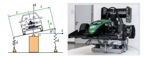
**5.** The figure shows a simplified idealization of a <u>commercial instrument</u> for measuring the inertial properties of large objects. It operates by measuring the amplitude and frequency of small oscillations of a platform, together with the horizontal and vertical reaction forces at the pivot.
