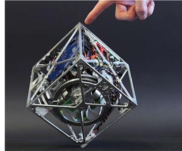
**Part 1:** Find formulas for the mass moments of inertia of the frame and the wheel (about the center of the wheel).
