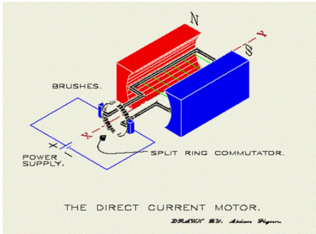
Power supply (e.g. Battery, or solar cell) applies voltage  $V$  to motor
