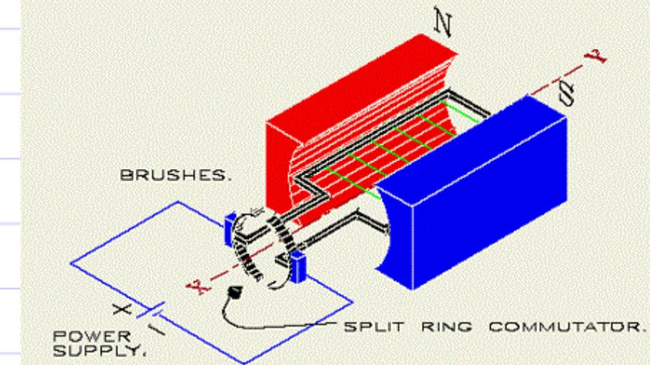
$$I = (V - \beta\omega)/R \quad T = \begin{cases} \beta I - T_0 - \gamma_0 \omega & \beta I > T_0 \\ 0 & \beta I < T_0 \end{cases}$$
