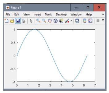
Here, x and y are just rows of numbers. MATLAB plots the graph by joining up successive pairs of x-y points with straight lines. For the plot to work, x and y must be vectors, and they must have the same length.
