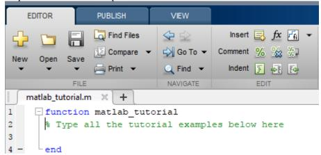
then save the file. Type all the examples that appear below between the 'function' and 'end' lines. It will be important to save most of the homeworks you do in ENGN40 as a function with this general format.
