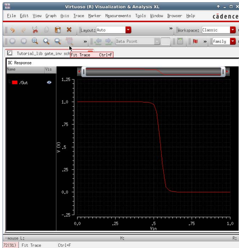
Figure 19 Output plot for a DC sweep analysis of a CMOS inverter
