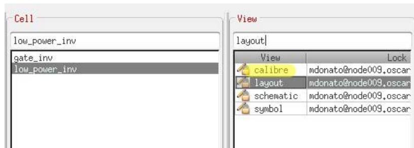
In order to simulate the new circuit with parasitics, go to ADE L (the setup for the simulation is the same as before in part 4). Before running the simulation, go to **Setup > Environment** and add calibre before the word schematic in Switch View List as shown in the figure below. Confirm and run the simulation.
