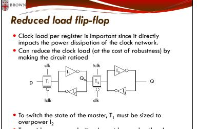
• To avoid reverse conduction,  $I_4$  must be weaker than  $I_1$ .
