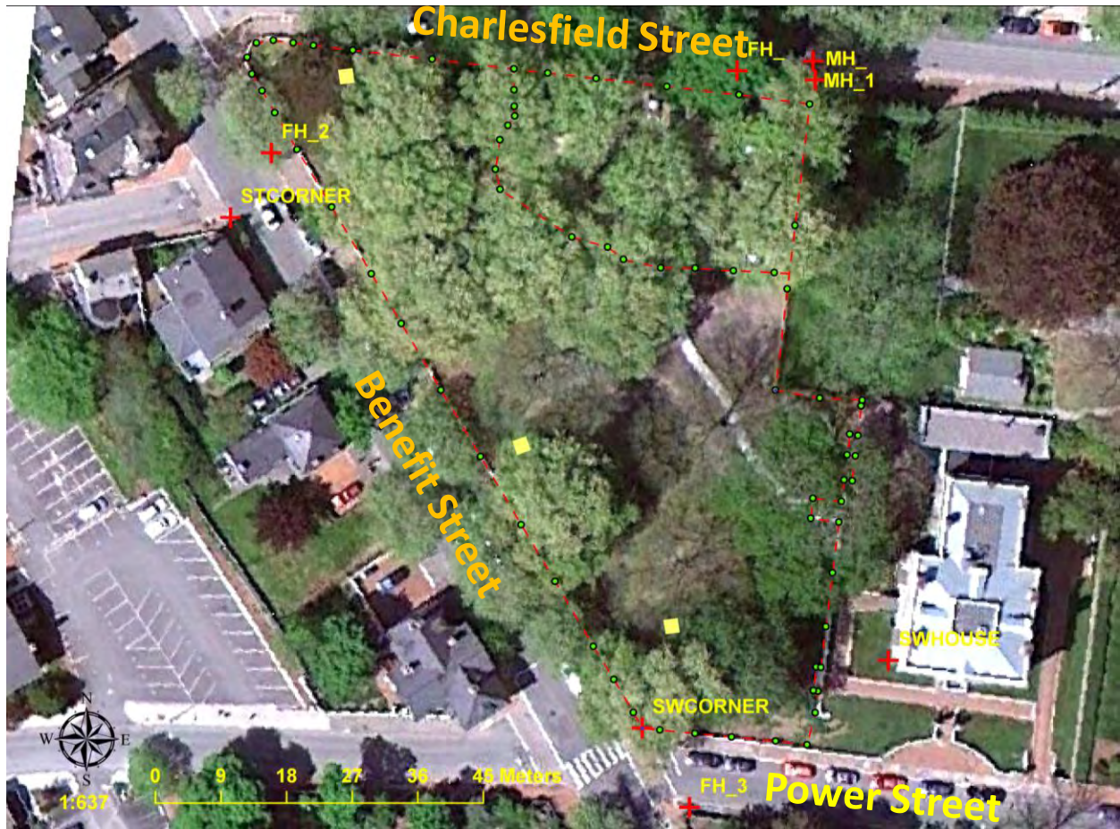
Figure 3: Satellite image overlaid on the GIS database. Outline points are visible as green dots connected by a dashed red line. Yellow squares correspond to units 10, 11, and 12 (South to North) and red crosses are georeference points (FH=Firehydrant, MH=Man Hole cover).
