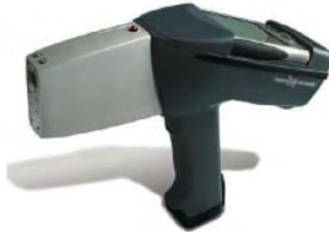
**Figure 3: Innov-X Alpha 4000 Handheld XRF**
