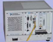
Fig 2. New PXI receiver, made by National Instruments, is lighter (16 lbs), smaller (26 cm x 21 cm x 18cm), and faster than prior hardware. It contains an embedded controller, which serves as a rugged internal computer, a digitizer to rapidly collect data, and a data acquisition board for slower input and output.
