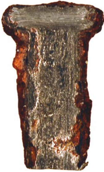
Figure 5. Specimen KR-1 - Interior of a machine-headed nail from Woodhouse, 19 th century (no magnification). The impact of the powerful mechanized heading process caused the regular and fairly even horizontal grain direction in the nail head.
