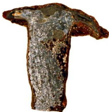
Figure 1. Specimen KR-20 - Old House hand wrought nail with high phosphorous content (hill and valley texture) indicating that the nail was produced from bog ore in an iron bloomery (no magnification).
