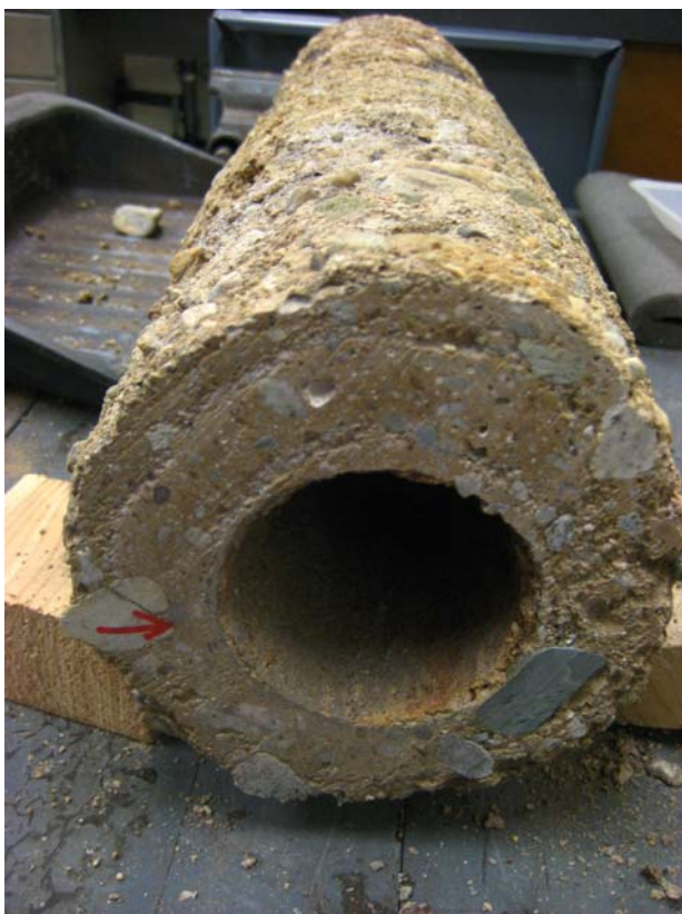
Figure 4. Tuyere cross section after cutting. Red arrow points to “bottom”, or portion that rested downwards. The interior of the bottom area had a residue buildup from use.
