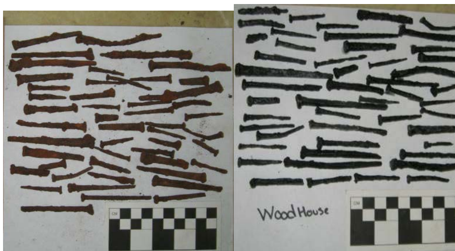
Woodhouse Nails Before and After Conservation (Miller 2007)
