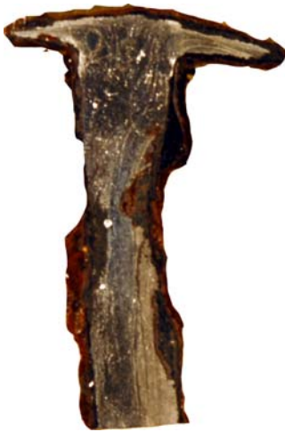
Figures 6 & 7. Specimen KR-10A – hand wrought nail from the Woodhouse, 17 th century. Fig. 6 (left) – no magnification, Fig. 7 (right)- 4x magnification photomosaic. Evidence of repeated impacts from and shaping by a blacksmith's hammering is clearly visible in the head, where the ferrite grains are tightly compressed at the tips of the head. The black lines and concentrations are dense slag deposits, indicating the impure and low quality of this nail, likely made in a bloomery from bog ore.
