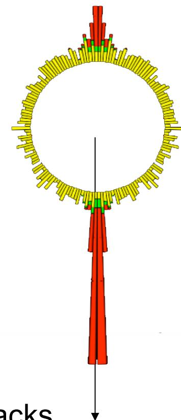
Even for asymmetric dijets, summing over tracks down to  $p_T$  of 500 MeV/c, the  $p_T$  balance is recovered
