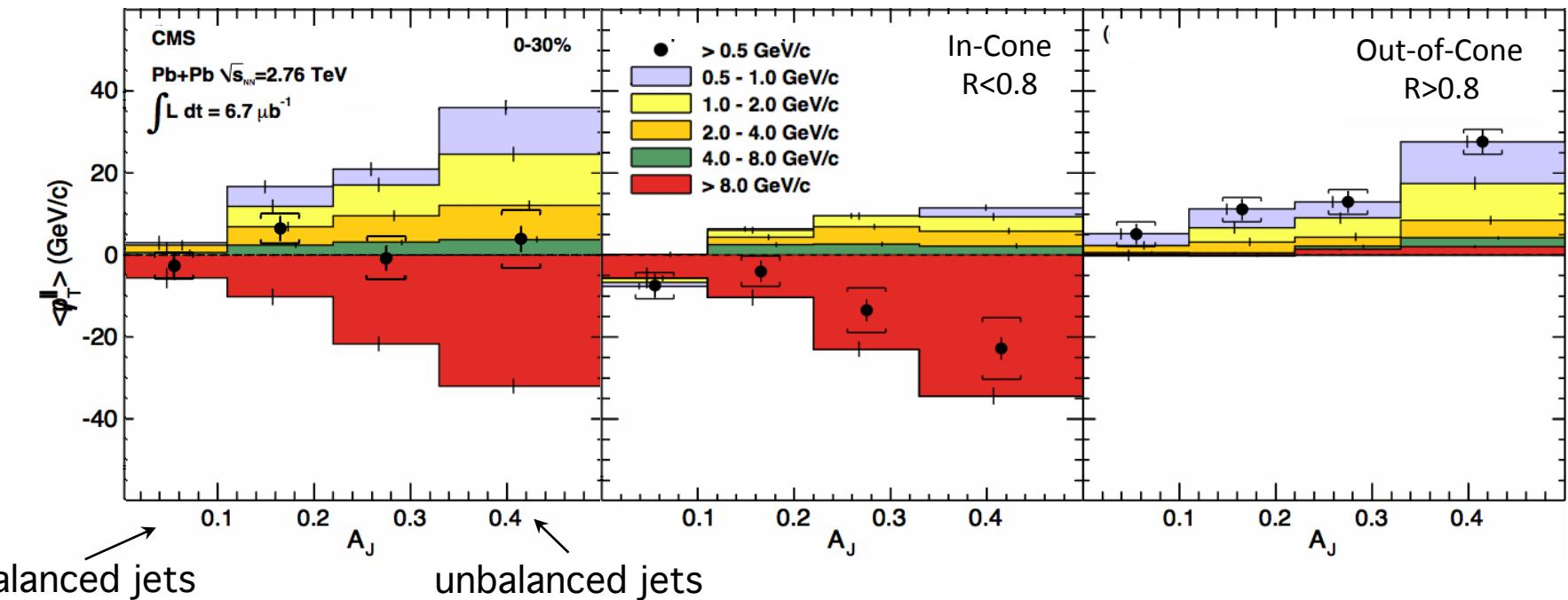
The lost energy carried by low  $p_T$  particles is mostly transferred to large angle with respect to the dijet
