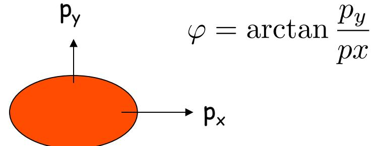
$$v_2 = \frac{\langle p_x^2 \rangle - \langle p_y^2 \rangle}{\langle p_x^2 \rangle + \langle p_y^2 \rangle}$$
