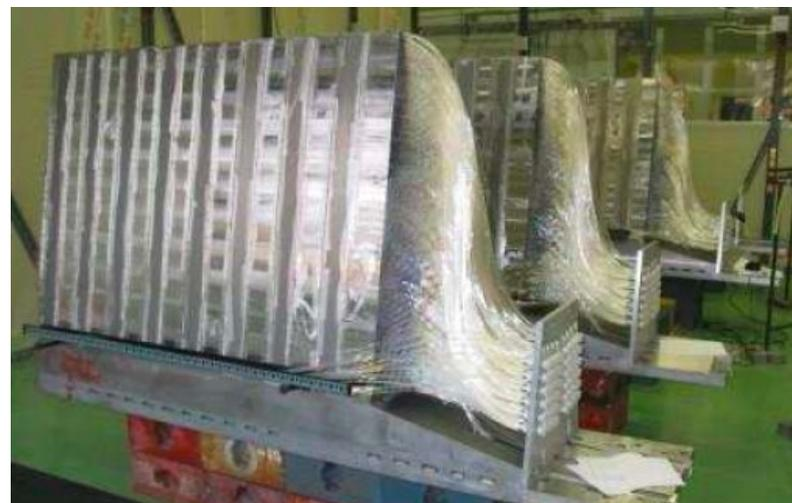
*Fiber read out connected to  $r\text{-}\Phi$  wedges.*
