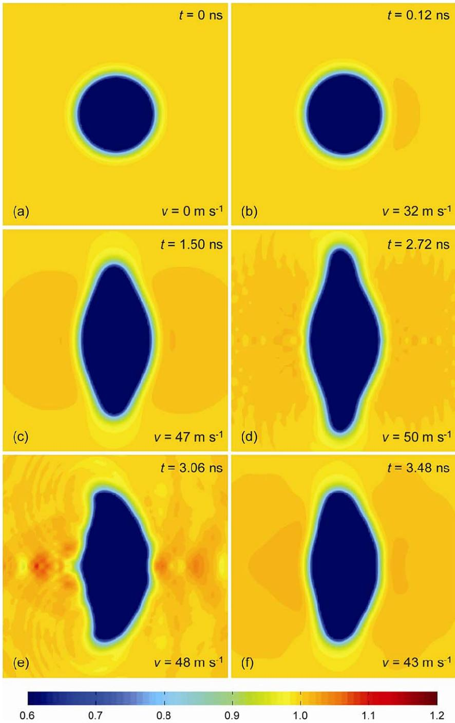
**Fig. 2** (Color online) Plot of the helium number density  $m_{\text{He}}|\psi|^2/\rho$  surrounding an electron bubble at different times. The side of each square is  $120 \text{ \AA}$ . The pressure  $P = 0$
