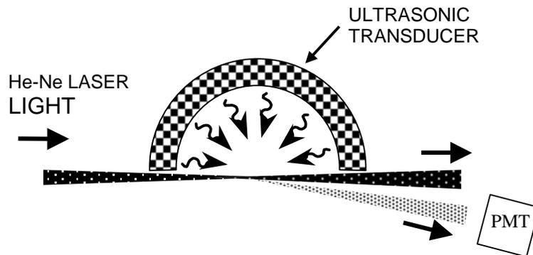
*Figure 3.* Schematic diagram of the experimental setup to study cavitation in liquid helium. Scattered laser light is detected by the photomultiplier (PMT).
