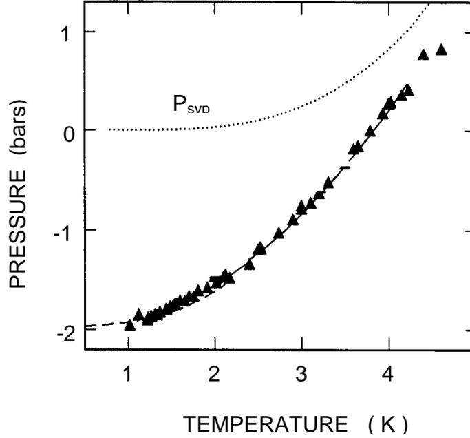
Figure 2. Negative pressure needed to explode an electron bubble in helium-4 as a function of temperature from ref. 23. The solid curve is from theory and the triangles are the measured values. The dotted line indicates the saturated vapor pressure.
