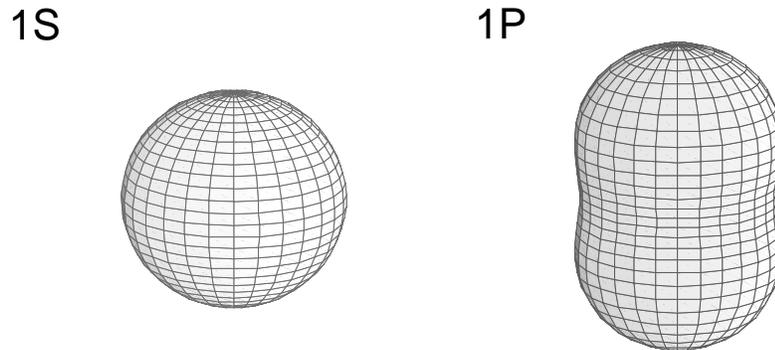
*Figure 7.* Equilibrium shape of electron bubbles with the electron in the 1S and the 1P states.
