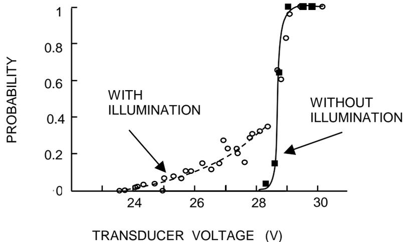
Figure 8. Probability of cavitation with and without illumination. Light produces bubbles containing 1P electrons which are more easily broken.
