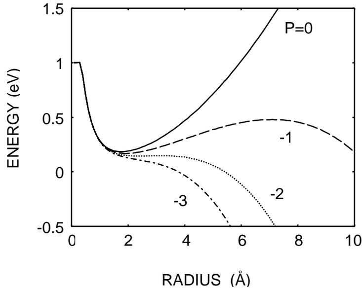
Figure. 1. Energy of an electron bubble as a function of the radius. The different curves are labeled by the pressure in bars.
