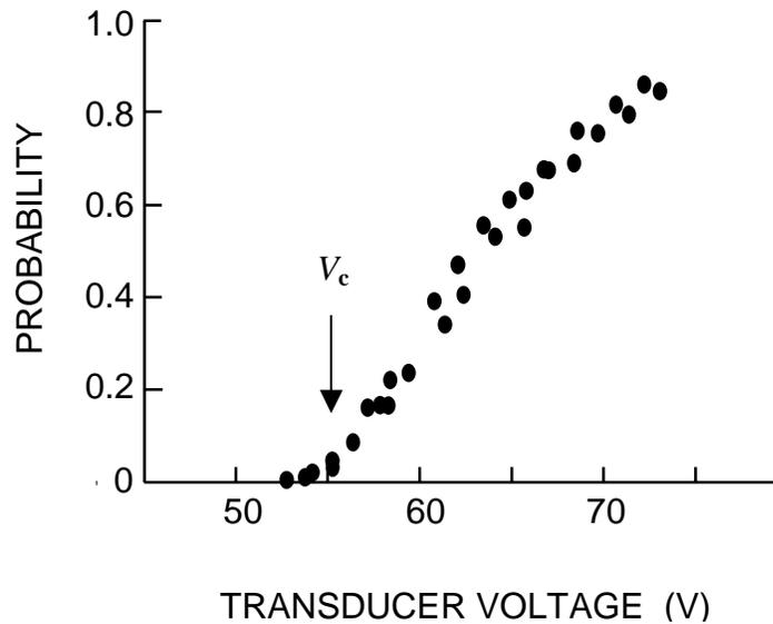
Figure 4. Example of the results from a measurement of the probability of cavitation as a function of applied transducer voltage.
