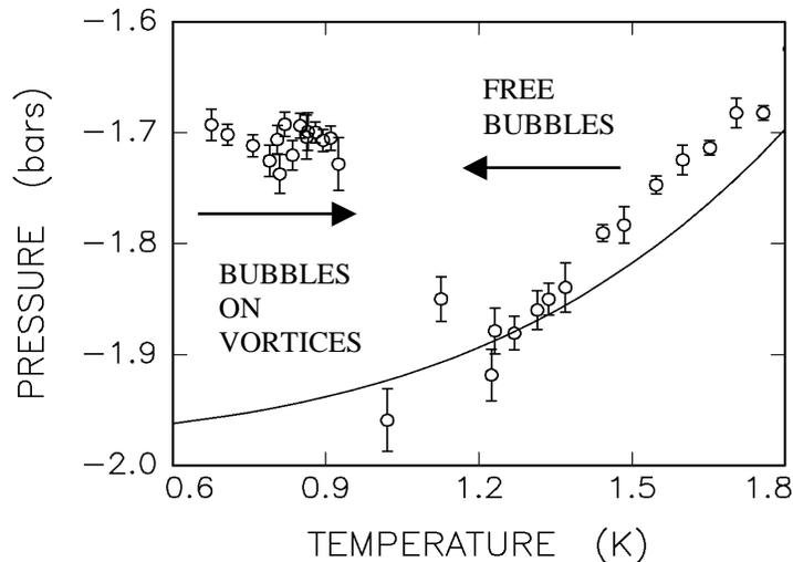
Figure 6. Critical pressure at which electron bubbles explode as a function of temperature from ref. [29]. The solid curve is the theory for a bubble in bulk liquid.
