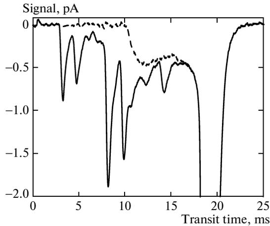
**Fig. 1.** Results from a time-of-flight mobility experiment performed at 0.991 K as reported in [22]. The solid curve shows the signal arriving at the collector as a function of time. The dashed curve is the signal after an algorithm has been used to remove the peaks. The length of the experimental cell is 6.15 cm and the drift field is  $82.1 \text{ V cm}^{-1}$ .
