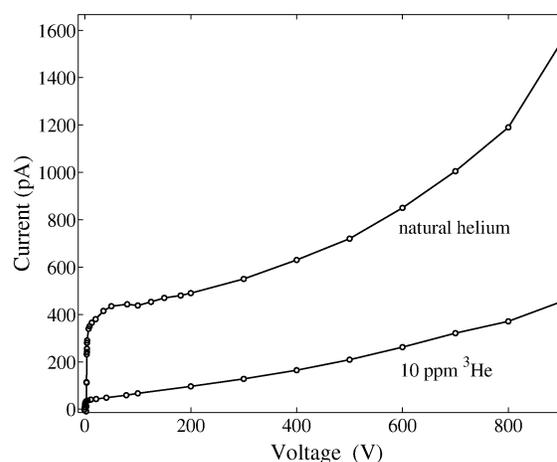
**FIGURE 2.** Current as a function of potential applied across the cell half full of helium. The sign of the potential is such that electrons travel upwards through the liquid and vacuum to the electrode on the top of the cell.
