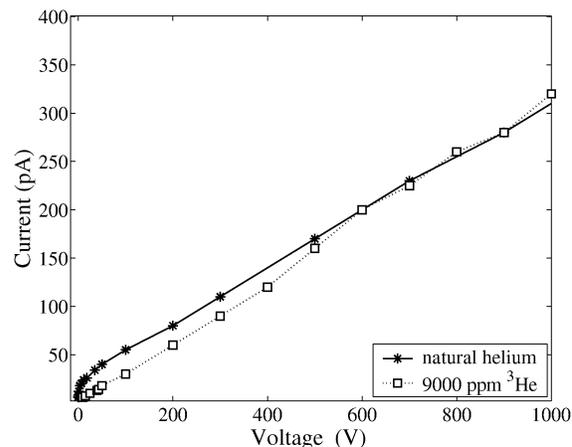
**FIGURE 1.** Current as a function of potential applied across the cell filled with natural helium and  $^4\text{He}$  with 0.9%  $^3\text{He}$ .
