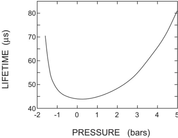
Fig. 7. Lifetime for radiative decay of the 1P state as a function of pressure.
