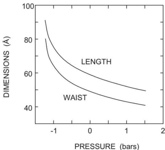
Fig. 4. Length and waist diameter of the 2P bubble as a function of pressure.
