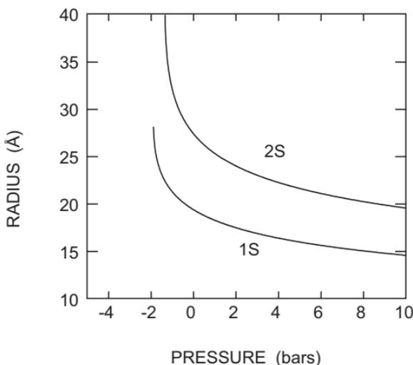
Fig. 5. Radius of the 1S and 2S bubbles as a function of pressure. The 1S and 2S bubbles become unstable at  $-1.89$  and  $-1.33$  bars, respectively.
