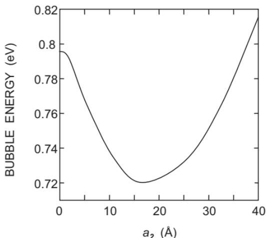
Fig. 12. The total energy of a two-electron bubble as a function of the parameter  $a_2$ . The distance from the center of the bubble to the surface in direction  $\theta$  is  $R + a_2 P_2(\cos \theta)$ , where  $R$  is  $34 \text{ \AA}$ .
