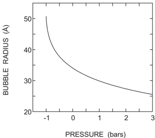
Fig. 11. The radius that minimizes the total energy of a two-electron bubble as a function of the pressure.
