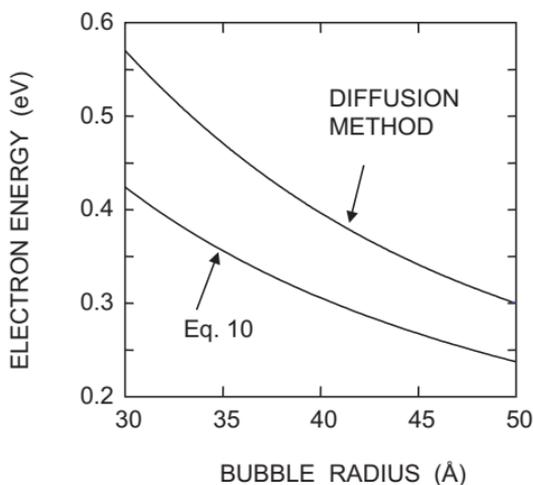
Fig. 9. Energy of two electrons inside a spherical bubble as a function of the bubble radius.
