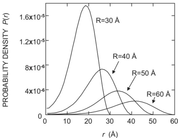
Fig. 10. Electron probability density as a function of distance  $r$  from the bubble center for a series of bubble of different radius  $R$ .
