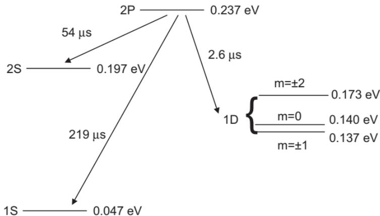
Fig. 8. Summary of the decay of the 2P bubble at zero pressure. The lifetime of the different decay channels and the energy of the different electron states inside the equilibrium 2P bubble shape are indicated.
