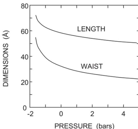
Fig. 2. Length and waist diameter of the 1P bubble as a function of pressure.
