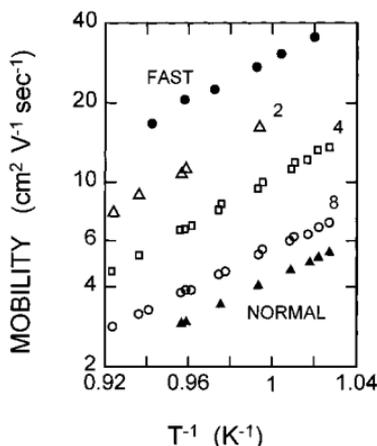
Fig. 11. Mobility of negative ions in superfluid helium plotted versus the inverse of the temperature. Solid triangles are for the normal electron bubble, open squares, circles and triangles are for three of the exotic ions, and solid circles are the fast ion. These data are taken from ref. 30.
