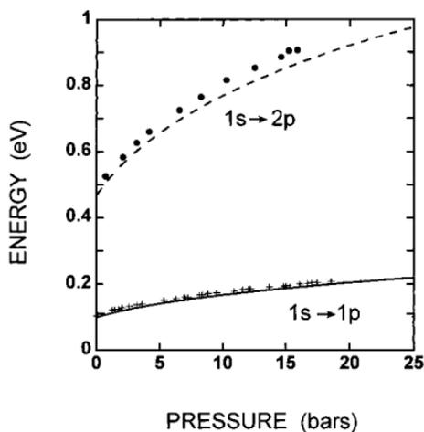
Fig. 3. Energy of the 1s → 1p and 1s → 2p transitions as a function of pressure. Solid curves show the results of the calculation described in the text. The crosses are the data points of Grimes and Adams, Ref. 10, and the circles the data of Zipfel, Ref. 12.
