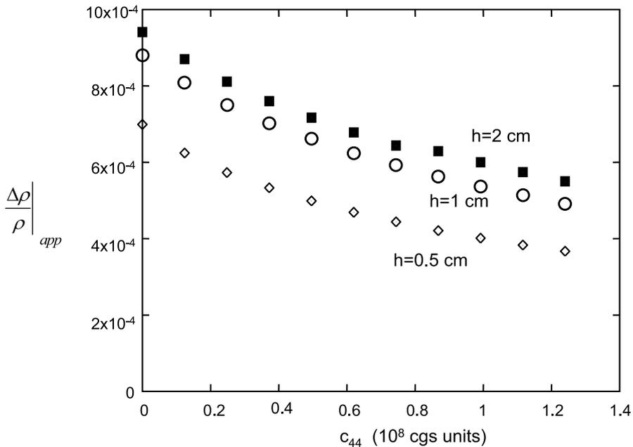
**Fig. 2** Apparent supersolid fraction  $(\delta\rho/\rho)_{app}$  for a single crystal of solid helium as a function of the value of  $c_{44}$ . The cell has a radius of 0.5 cm and a height  $h$  as indicated in the figure. Results are for a crystal with  $c$ -axis perpendicular to the rotation axis of the oscillator
