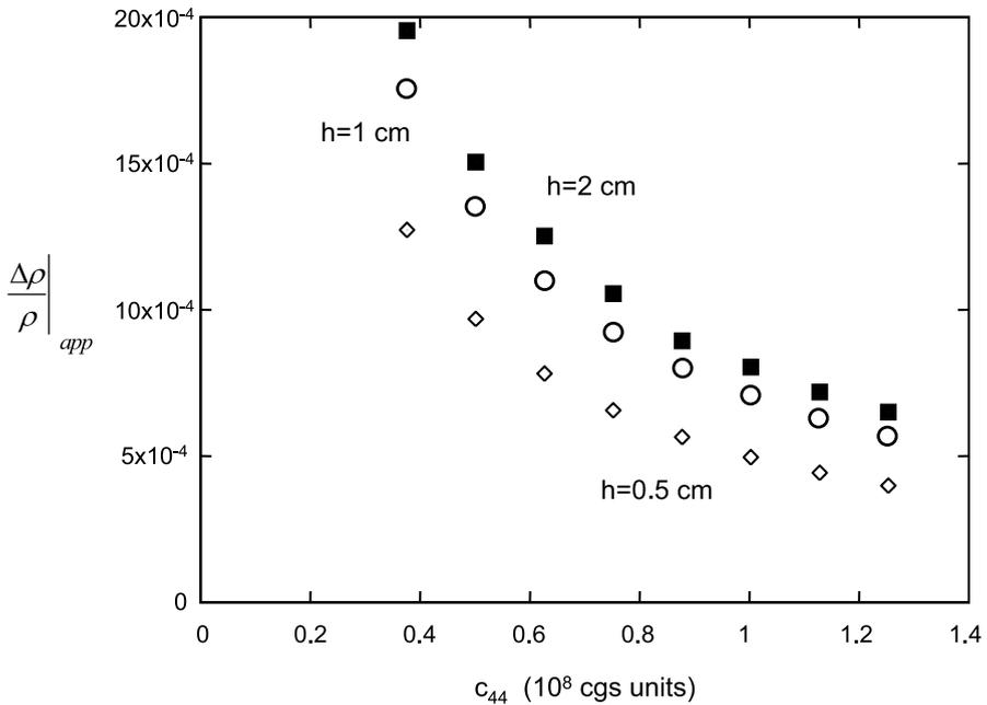
**Fig. 3** Apparent supersolid fraction  $(\delta\rho/\rho)_{app}$  for polycrystalline solid helium as a function of the value of  $c_{44}$ . The radius of the cell is 0.5 cm and a height  $h$  as indicated in the figure
