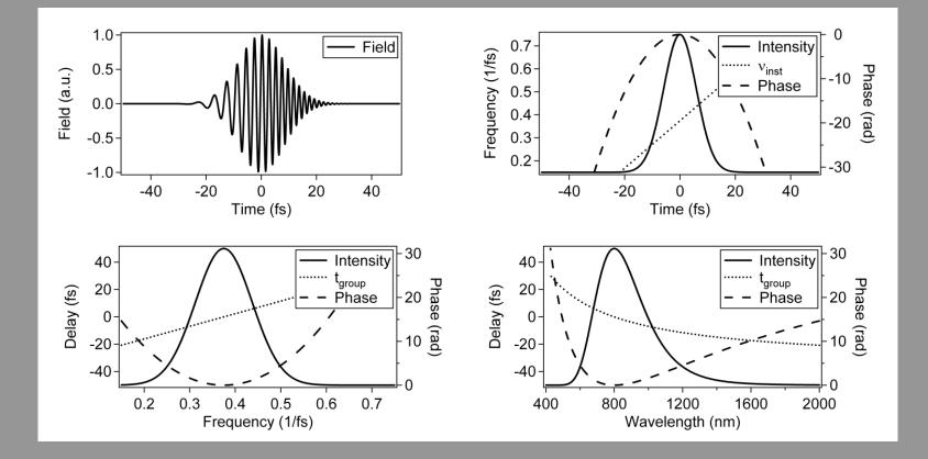
Here the quadratic phase has stretched what would have been a 3-fs pulse (given the spectrum) to a 13.9-fs one.
