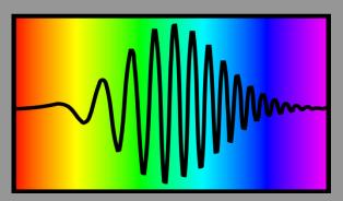
$$\mathscr{C}(t) \propto E_0 \exp\left[-\alpha t^2\right] \exp\left[i\left(\omega_0 t + \beta t^2\right)\right] + c.c \quad \text{where } \alpha \propto \left(1/\tau_G\right)^2$$
