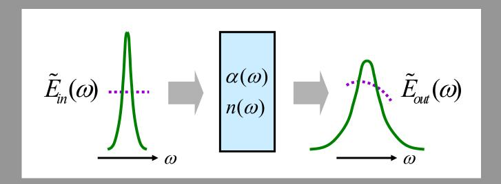
$$\tilde{E}_{out}(\omega) = \tilde{E}_{in}(\omega) \exp[-\alpha(\omega)L/2] \exp[-in(\omega)kL]$$
