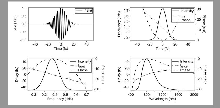
As with positive chirp, the quadratic phase has stretched what would have been a 3-fs pulse (given the spectrum) to a 13.9-fs one.
