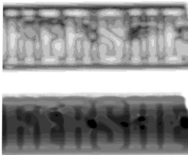
Fig. 4. Two THz images of a chocolate bar. The upper image shows the variation in amplitude of the transmitted waveform. Here, the embossed lettering is only visible because of scattering effects at the stepped edges of the embossing, whereas the almonds are clearly visible due to their stronger absorption of the radiation. The lower image shows the variation in transit time of the THz pulse, reflecting the accumulated phase. Here, the almonds are almost invisible, but the variation in the thickness of the sample is quite clear, allowing the embossed lettering to be easily discerned. The darkest spots on the lower image represent regions where the amplitude of the transmitted pulse was too small to make an accurate determination of the transit time
