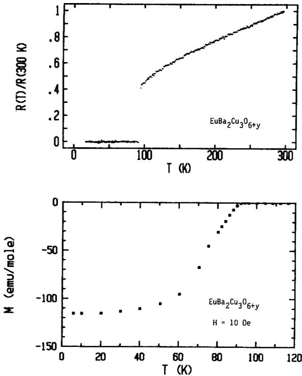
Fig.1 Resistivity and magnetization at  $H = 10$  Oe as a function of temperature for  $\text{EuBa}_2\text{Cu}_3\text{O}_{6+y}$
