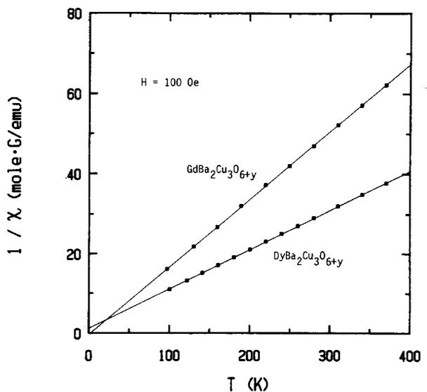
Fig.2 Linear temperature dependence of the inverse susceptibility ( $H = 100$  Oe) for  $\text{Gd}\text{Ba}_2\text{Cu}_3\text{O}_{6+y}$  and  $\text{Dy}\text{Ba}_2\text{Cu}_3\text{O}_{6+y}$
