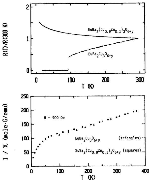
Fig.3 Resistivity versus temperature for  $\text{EuBa}_2(\text{Cu}_{0.9}\text{Zn}_{0.1})_3\text{O}_{6+y}$ , compared with  $\text{EuBa}_2\text{Cu}_3\text{O}_{6+y}$ . Note the complete suppression of superconductivity by 10% Zn-substitution. The squares and triangles are the inverse susceptibility data for  $\text{EuBa}_2(\text{Cu}_{0.9}\text{Zn}_{0.1})_3\text{O}_{6+y}$  and  $\text{EuBa}_2\text{Cu}_3\text{O}_{6+y}$  respectively. The magnetic behavior remains the same above  $T = 100\text{ K}$ .
