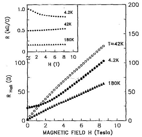
FIG. 2. Hall resistance curves of the 9 nm-(In,Mn)As/GaSb heterostructure at different temperatures. Mn fraction is  $x \sim 0.10$ . Inset figure shows magnetoresistance curves.
