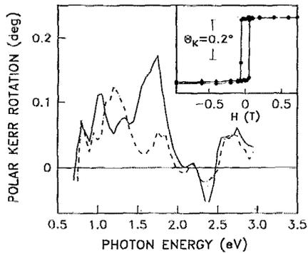
FIG. 3. Remanent polar Kerr rotation spectra at 5.5 K for two heterostructures with different structural parameters: 9 nm-(In,Mn)As/136 nm-AlSb with  $x=0.1$  (solid line), and 19 nm-(In,Mn)As/195 nm-AlSb with  $x=0.07$  (dashed line). Curie temperatures are  $T_C \sim 35$  and 17 K, respectively. Inset figure shows a square hysteresis loop at  $h\nu=1.75$  eV.
