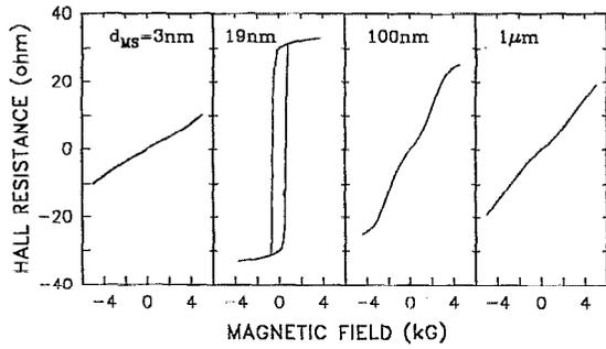
FIG. 1. Development of square loop hysteresis in the Hall resistance as a function of (In,Mn)As layer thickness  $d_{MS}$  in  $p$ -(In,Mn)As/AlSb heterostructures. Mn fraction is  $x \sim 0.07$ , and  $T = 4.2$  K.
