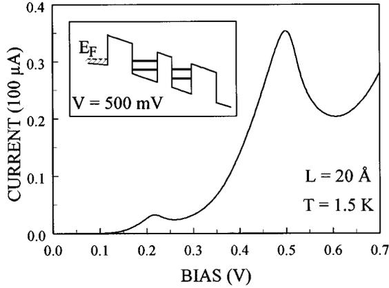
FIG. 1. Tunneling  $I(V)$  characteristics at  $T=1.5$  K of triple-barrier RTS's with a middle-barrier width  $L=20$  Å. The inset gives the self-consistent potential distribution for  $V=500$ -mV applied bias, indicating  $HH_0$  and  $LH_0$  energy subbands in each well calculated in the absence of interwell coupling.
