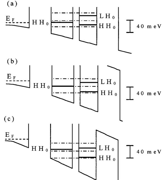
FIG. 3. Schematic valence-band diagrams of triple-barrier RTS's with a middle-barrier width  $L=10$  Å at bias values corresponding to the experimentally measured resonances: (a)  $V=175$  mV, (b)  $V=265$  mV, and (c)  $V=345$  mV. The dash-dotted line represents the double-well tunneling subbands. The  $LH_0$  subband in the first well, which lies  $\sim 35$  meV above the  $HH_0$  subband in the same well, has been omitted for clarity.
