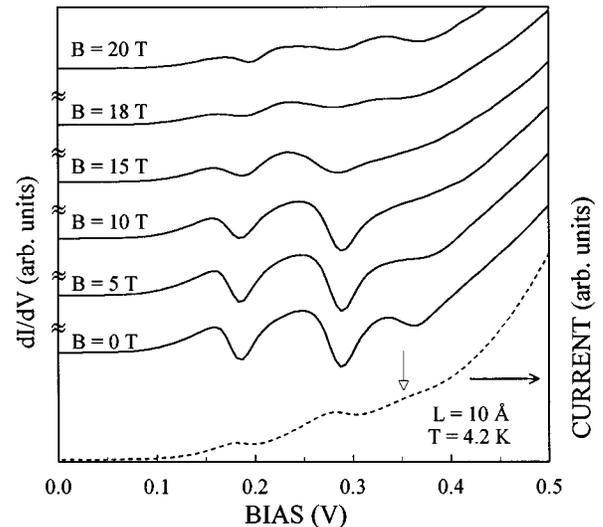
FIG. 4. Conductance  $dI/dV$  characteristics of the  $L=10\text{-}\text{\AA}$  triple-barrier RTS's at  $B_\parallel=0, 5, 10, 15, 18,$  and  $20$  T. The dashed curve indicates  $I(V, B_\parallel=0)$  for comparison, with the open arrow indicating the  $\text{HH}_0^{(1)}\text{-LH}_0^{(2)}$  resonance. The curves have been shifted for clarity.
