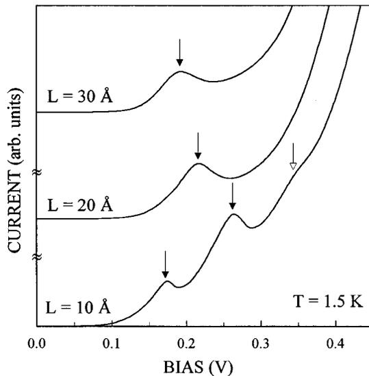
FIG. 2. Tunneling  $I(V)$  characteristics at  $T=1.5$  K of triple-barrier RTS's in the low-bias range for  $L=10$ , 20, and 30 Å. The  $I(V)$  curves of the different structures have been rescaled and shifted for clarity. Solid arrows delineate the observed peak positions of the  $HH_0^{(1)}$ - $HH_0^{(2)}$  resonances, and the open arrow delineates the  $HH_0^{(1)}$ - $LH_0^{(2)}$  resonance.
