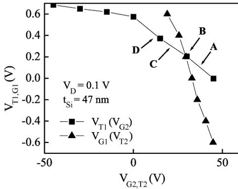
Fig. 3. Front-channel threshold voltage versus back-gate bias  $V_{T1}(V_{G2})$  and back-channel threshold voltage versus front-gate bias  $V_{G1}(V_{T2})$  for a 47-nm-thick transistor ( $L = 10 \mu\text{m}$ ,  $W = 10 \mu\text{m}$ ).
