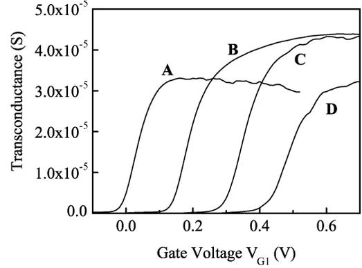
Fig. 4. Transconductance versus front-gate voltage for 47-nm-thick transistor ( $L = 10 \mu\text{m}$ ,  $W = 10 \mu\text{m}$ ) in the virtual DG mode: the offset voltages  $V_{T1,2}$  in (1) correspond to points A, B, C, and D shown in Fig. 3.
