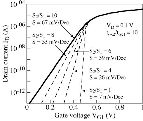
Fig. 2. Simulations using (1) for  $t_{ox2}/t_{ox1} = 10$  (i.e.,  $\Delta V_{G2} = 10 \Delta V_{G1}$ ) and various  $S_2/S_1$  ratios. These curves have been obtained by using the model described reference [5] and by considering two independent channels (front and back). Only the bold curve is correct because for  $S_2/S_1 = t_{ox2}/t_{ox1} = 10$ , equation (1) is identical to the accurate (2).
