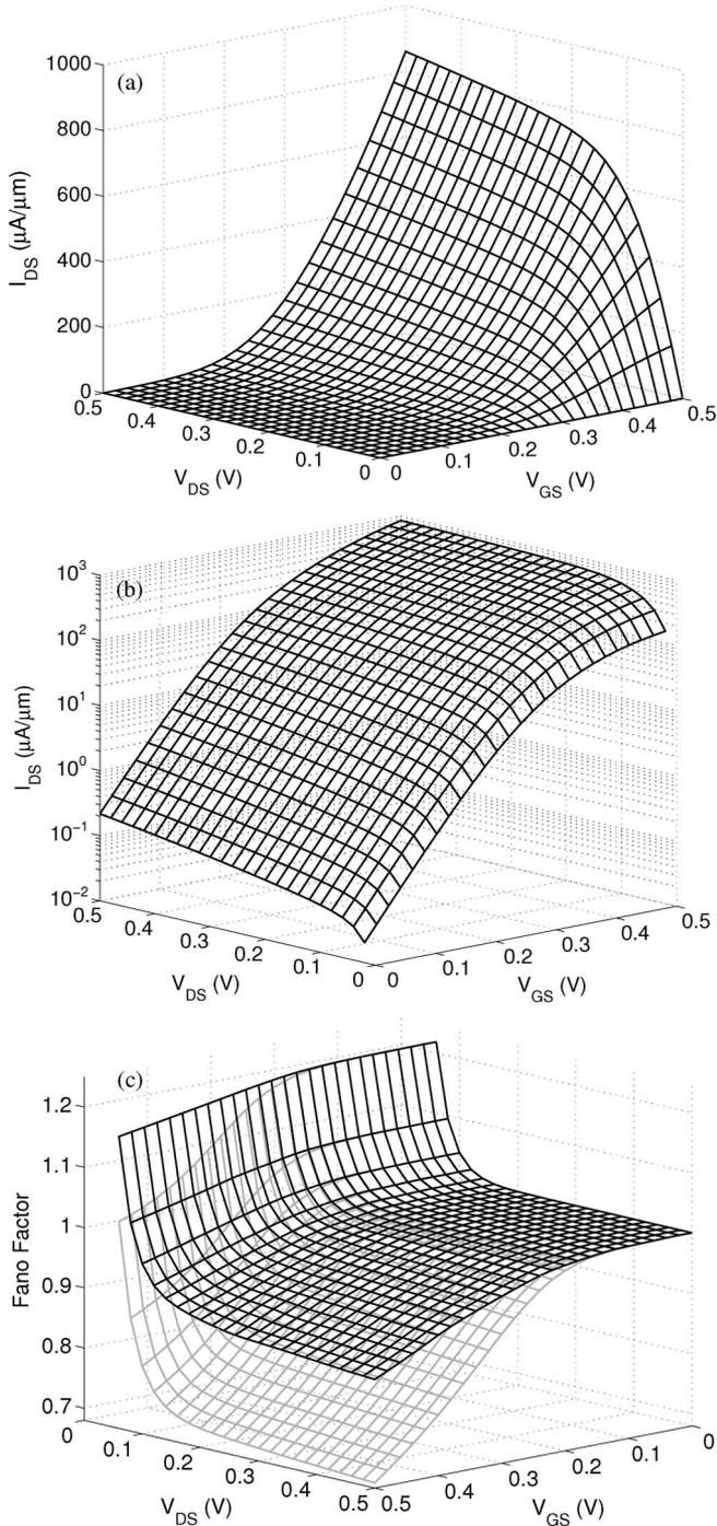
Fig. 2.  $I$ - $V$  and noise characteristics for a DG-MOSFET with  $L_G = 10$  nm and Si channel thickness of 5 nm, calculated using a 2-D Schrödinger-Poisson solver. The  $x$  and  $y$  axes represent the  $V_{GS}$  and  $V_{DS}$ , and the  $z$ -axis represents (a) the current in linear scale, (b) the current in logarithmic scale, and (c) the Fano factor in a fully ballistic case (shown in gray) and with LA scattering effects turned on (shown in solid black).
