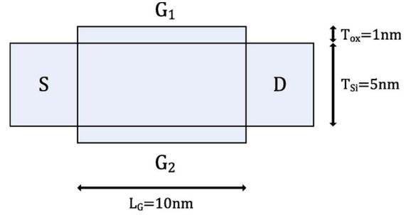
Fig. 1. Schematic of an ITRS-predicted LSTP DG-MOSFET with an effective gate length of  $L_G = 10$  nm, Si channel thickness of  $T_{\text{Si}} = 5$  nm, and equivalent oxide thickness of  $T_{\text{ox}} = 1$  nm.
