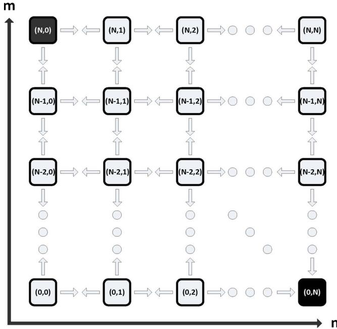
Fig. 4. Two-dimensional Markov chain for a flip-flop. Each axis labels different states corresponding to different voltages on capacitors  $C_1$  and  $C_2$ .
