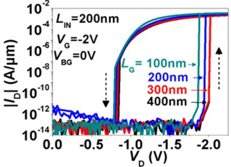
Fig. 7 Experimental  $I_D$ - $V_D$  curves for the  $Q_S$ -operated devices with different  $L_G$ . The  $|V_{ON}|$  decreases slightly as  $L_G \leq 300nm$ .
