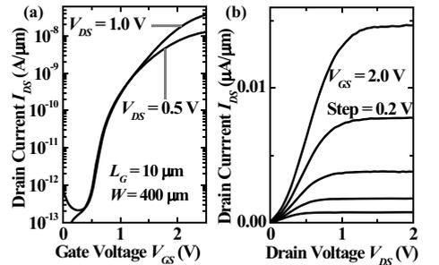
Fig. 4. (a) Measured  $I_{DS}-V_{GS}$  and (b)  $I_{DS}-V_{DS}$  curves of a typical  $nTFET$ . All devices used in this study have a  $L_G/W$  of  $10 \mu m/400 \mu m$ .
