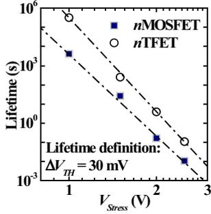
Fig. 10. PBTI lifetime projection of  $nTFET$  and  $nMOSFET$ , showing that  $nTFET$  has a longer lifetime than  $nMOSFET$  at all PBTI stresses.
