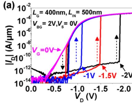
Fig. 4 Experimental  $I_D$ - $V_D$  curves of the devices operating with (a)  $V_{BG}$  and (b)  $Q_S$ , respectively, showing sharp switching and hysteresis, indicated by the dashed arrows.
