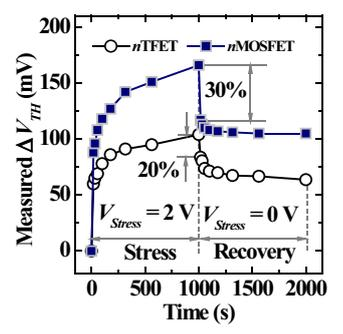
Fig. 8.  $\Delta V_{TH}$  evolution in stress phase and recovery phase. An initial recovery in the first 18 seconds of  $nTFET$  is 20%, which is lower than that of  $nMOSFET$ .
