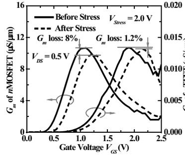
Fig. 11.  $G_m-V_{GS}$  curves of  $nTFET$  and  $nMOSFET$  before and after PBTI stress at  $2.0$  V. The data were obtained from the curves shown in Fig. 5.
