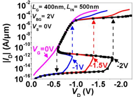
Fig. 5 Simulated  $I_D$ - $V_D$  reproduces the experimental data in Fig. 4(a). Dots show the simulation with impact ionization turned on.
