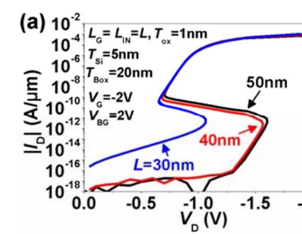
Fig. 8 Simulation is conducted to study the scaling capability of  $V_{BG}$ -operated  $Z^2$ -FET. Note that  $L_G = L_{IN} = L$ . (a) The simulated  $I_D$ - $V_D$  curves show that the  $|V_{ON}|$  is not affected by  $L$  until it decreases to 30nm. (b) The dependence of  $|V_{ON}|$  on  $L$  reveals that the device can be scaled down to 35nm keeping the  $|V_{ON}| > 1.5V$ . The inset shows the simplified device structure used in simulation.
