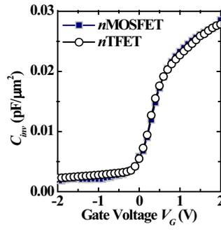
Fig. 7. Measured  $C_{inv}-V_G$  curves of a pair of fresh  $nTFET$  and  $nMOSFET$ . The impact of the narrow TJ region (several nm) on  $nTFET$   $C_{inv}$  is negligible. For a given  $V_G$ ,  $nTFET$  and  $nMOSFET$  have the same  $Q_{inv}$  and the same vertical field in  $HfO_2$  above the channel region.
