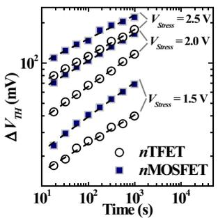
Fig. 9.  $\Delta V_{TH}$  versus stress time characteristics for  $nTFET$ s and  $nMOSFET$ s at different PBTI stresses, showing a power law dependence.
