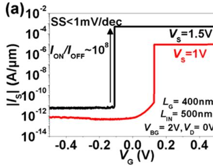
Fig. 2 Experimental  $I_S$ - $V_G$  curves of the devices operating with (a)  $V_{BG}$  and (b)  $Q_S$ , schematically shown in Fig. 1(a) and (b). Note the zero SS in both variants of the  $Z^2$ -FET.
