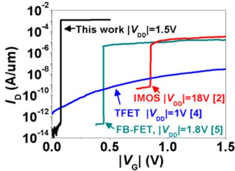
Fig. 3 Comparison between  $Z^2$ -FET and other sharp-switching devices.
