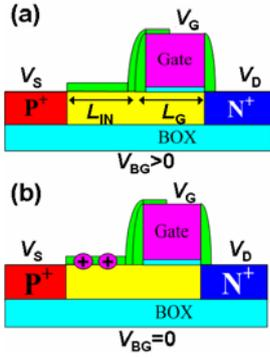
Fig. 1 Schematic view of the structure of  $Z^2$ -FETs operating with (a) backgate voltage ( $V_{BG}$ ) and (b) surface charge ( $Q_S$ ) on  $L_{IN}$  region.
