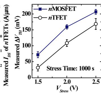
Fig. 6.  $\Delta V_{TH}$  of  $nTFET$ s and  $nMOSFET$ s at different PBTI stresses.  $V_{TH}$  of  $nTFET$  and  $nMOSFET$  is extracted for  $V_{GS}$  at  $I_{DS} = 1$  nA/ $\mu m$  and  $1 \mu m/400 \mu m$ , respectively, measured at  $V_{DS} = 0.5$  V.
