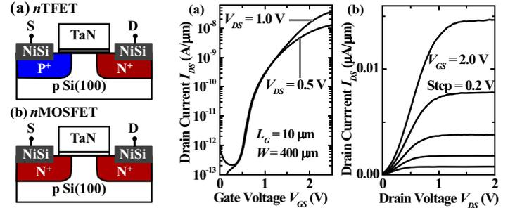
Fig. 3. Schematics of (a)  $nTFET$  and (b)  $nMOSFET$ .
