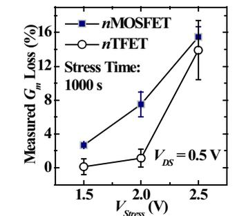
Fig. 12.  $nTFET$ s demonstrate less degradation of peak  $G_m$  as compared to  $nMOSFET$  at all PBTI stresses. The data were obtained at  $V_{DS} = 0.5$  V.
