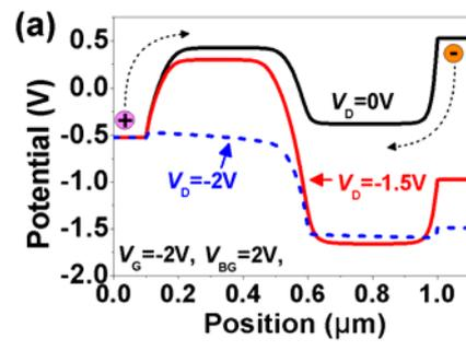
Fig. 6 (a) Simulated surface potential of the device under different  $V_D$ , showing that the carrier injection barriers under low  $|V_D|$  is eliminated at  $V_D = -2V$ . (b) The evolution of the  $V_n$  and  $V_p$  as  $|V_D|$  increases.
