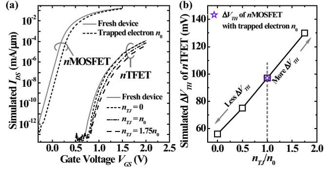
Fig. 2. (a) Simulated  $I_{DS}-V_{GS}$  curves of  $nMOSFET$  and  $nTFET$  with and without trapped electrons. Trapped electrons in  $HfO_2$  above TJ have a large impact on  $\Delta V_{TH}$  of  $nTFET$ . (b) If  $n_{TJ} < n_0$ ,  $nTFET$  has smaller  $\Delta V_{TH}$  compared to  $nMOSFET$ . Otherwise  $nTFET$  has larger  $\Delta V_{TH}$ .
