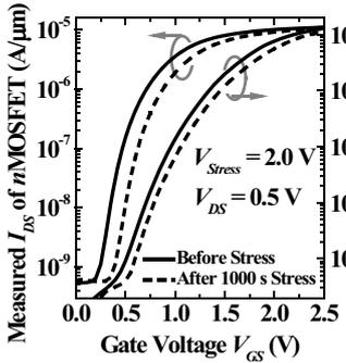
Fig. 5. Measured  $I_{DS}-V_{GS}$  curves of a pair of  $nTFET$  and  $nMOSFET$ s before and after PBTI stress at  $2.0$  V.  $nTFET$  has a smaller threshold voltage shift after the PBTI stress compared to  $nMOSFET$ .
