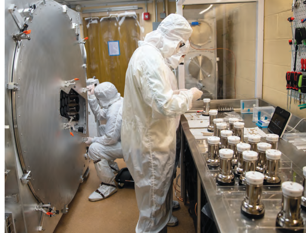
Researchers at Brown assembled in a special cleanroom an array of powerful light sensors to keep watch on the LUX-ZEPLIN dark matter detector in South Dakota.
