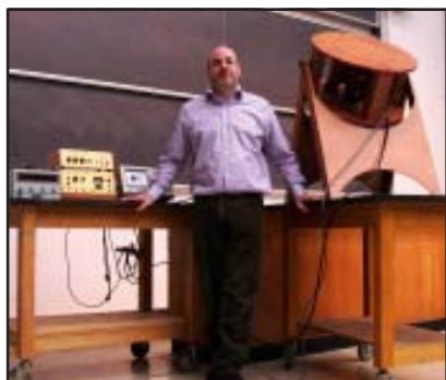
Jerry Zani with our newly acquired Earth's Field NMR device. With this apparatus students can observe the basic principles of NMR in the classroom.
